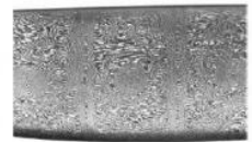
Blade has a ladder and rose pattern The inside of a Damascus blade, showing the carbide particles aligned as rows
